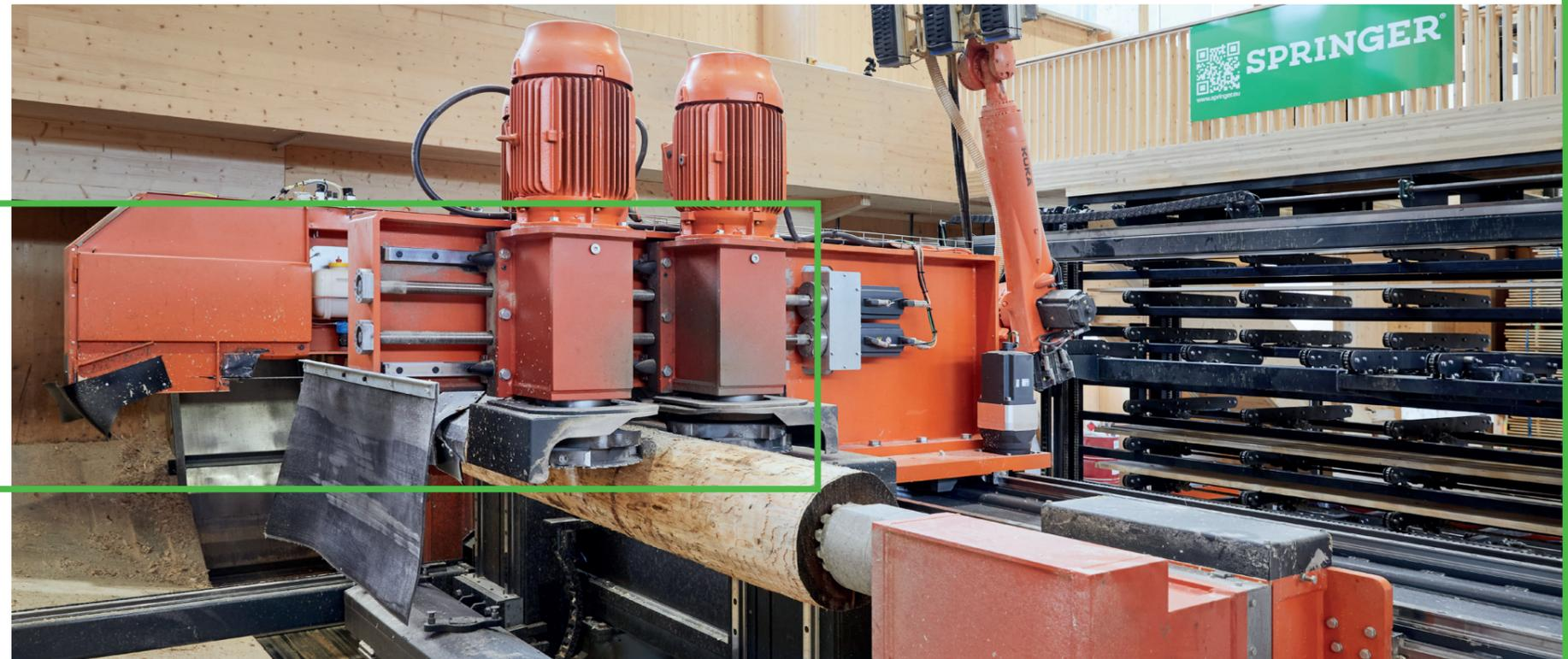
The SAWBOX redefines standards for log production. Its compact design centralizes all processing steps in one center, ensuring efficient production with minimal space needs. Unlike traditional sawmills, it streamlines processing into a single step, allowing for efficient production with only one operator.
